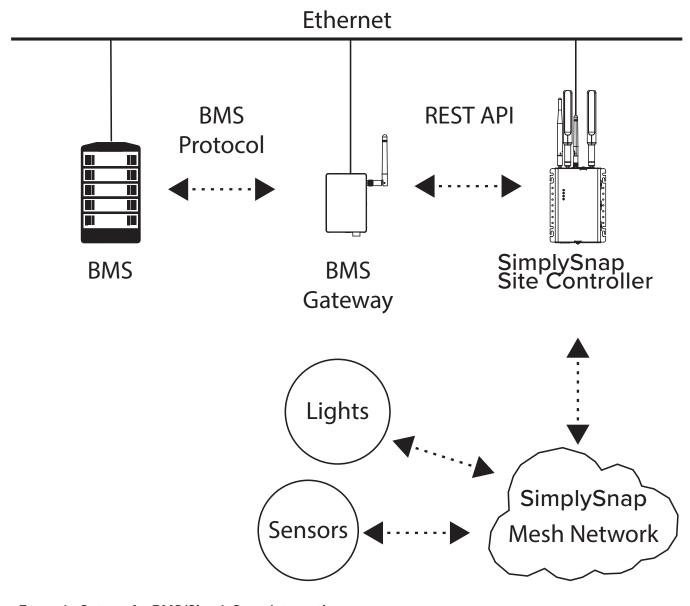
Example Setup of a BMS/SimplySnap Integration
