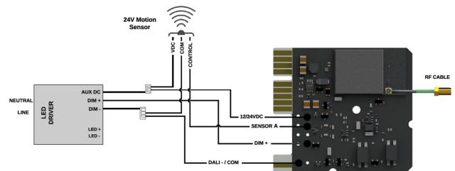
Figure 2 - Dim to OFF Wiring Diagram **WARNING:** · If a single Synapse controller is used to drive the DIM+ input of multiple LED drivers, then all of the DIM- lines from all drivers MUST be directly tied/shorted together to provide a common return/ground to the controller. 24V Motion · Synapse will not warranty or be liable for designs with Sensor any other electronic means of coupling DIM- lines from multiple drivers. RF CABLE AUX DC NEUTRAL DALI+ LED DALI -LINE LED+ LED -DALI - / COM
