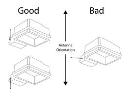
Figure 1 - Proper External Antenna Installation
