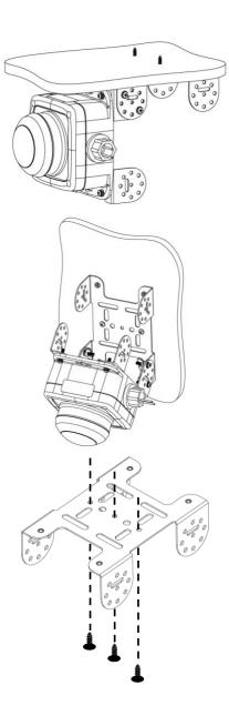
The drawings below demonstrate how to assemble the bracket so that the sensor is positioned at  $90^{\circ}$  relative to the mounting surface.
