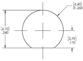
Figure 2 – Recommended mounting hole for 1/4-36UNS-2A threaded antenna
