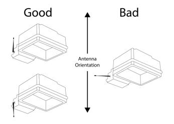
Figure 1 - Proper Antenna Installation
