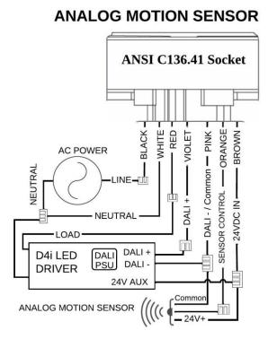
Figure 1 – C136-41 Socket Wiring Details
