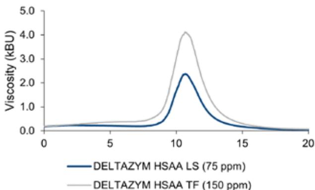
**Figure 1** - Viscosity profile during starch liquefaction (30% dry substance wheat flour, pH 4.5) of DELTAZYM® HSAA LS at half dose of DELTAZYM® HSAA TF. Initial, peak and final viscosity are significantly reduced, improving the liquefaction process and economics or allowing for further dose reduction.
