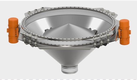
Bin Activators are commonly used to aid discharge of products where vessel geometry is compromised. Using vibration and applying this directly into the bulk solid material they aid flow and discharge of granular and powdered products from silos and hoppers.
