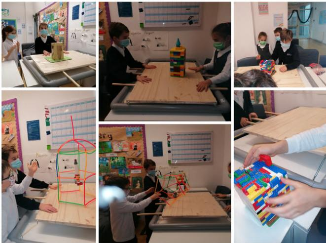
We found that it was the ones that used base isolations, a tuned mass damper (a pendulum) and controlled rocking, that worked the best.
