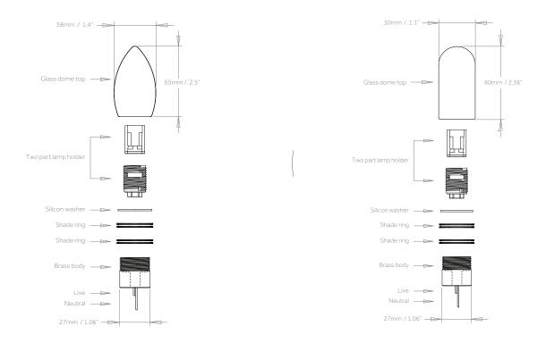
4) The glass shade is unscrewed to insert a G9 x 40 watt max halogen lamp.
