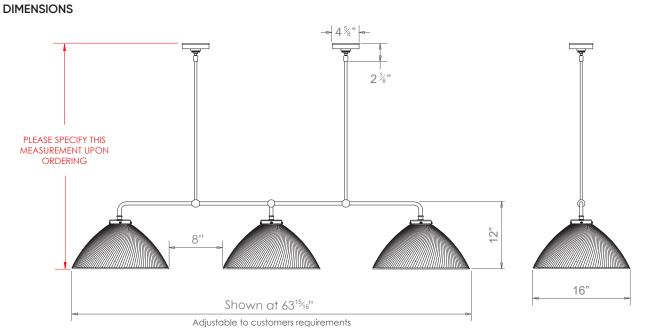
\*The electrical cable will exit from one side of the fixture.
