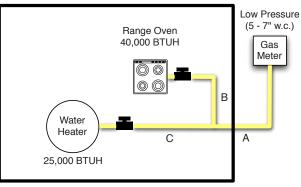
Figure 3.5 Low Pressure System—Series Arrangement
