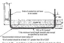
Figure 4.28 Installation in Nonmetallic Conduit Under Slab
