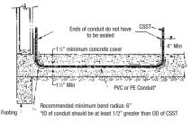
Figure 4.29 Installation in Nonmetallic Conduit In Slab
