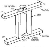
Figure 4.5 Holes and Cuts in Top and Sole Plates
