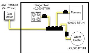
Figure 3.3 A low pressure parallel layout
