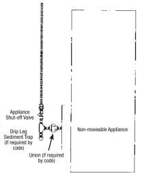
Figure 4.17 Direct Connection to Fixed Appliance
