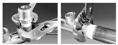
Figure 4.3 Supporting Manifold When Attaching Fittings
