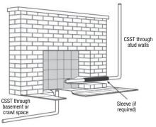
Figure 4.23 Routing to Masonry Fireplace
