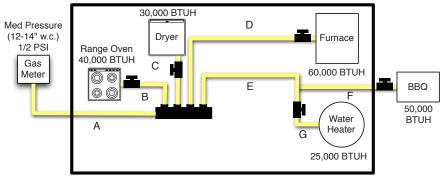
Figure 3.8 Medium Pressure System—Parallel Arrangement with Series Branch
