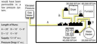
Figure 3.6 Medium Pressure System—Parallel Arrangement
