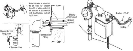
Figure 4.14 Connection to Building supported Meter
