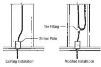
Figure 4.9 Extension of Existing Tubing Run
