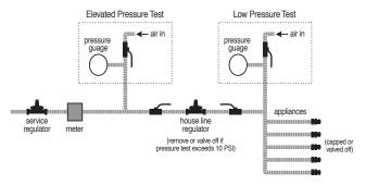
Figure 6.1 Pressure Test Requirements for a 2 PSI System
