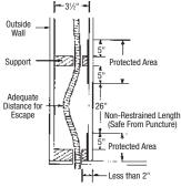
Figure 4.10 Elevated View of Unsupported Horizontal Tubing Run
