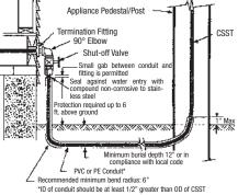
Figure 4.22 Fixed Outdoor Appliance (Underground Routing)
