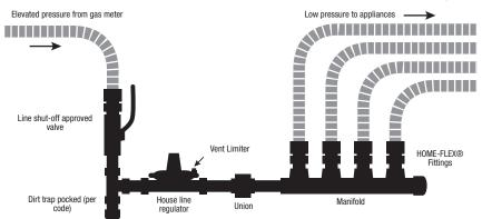
Figure 4.25 Example of Manifold Station Layout
