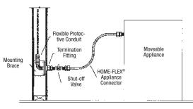
Figure 4.16 HOME-FLEX<sup>®</sup> Connection to Movable Gas Appliance
