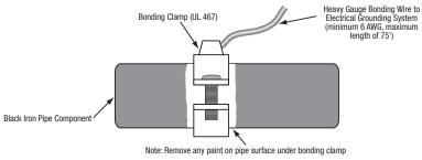
Figure 4.31 Bonding Connection to Rigid Black Iron Pipe
