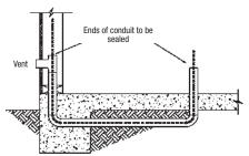
Figure 4.27 Installation in Nonmetallic Conduit with Venting
