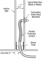
Figure 4.12 Use of Flexible Protective Conduit
