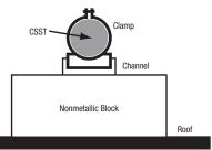
Figure 4.19 Rooftop Support with Strut
