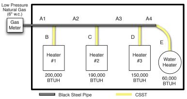
Figure 3.9 Low Pressure Hybrid System—Series Arrangement
