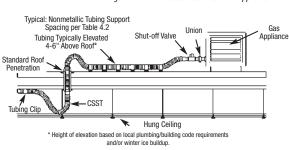
Figure 4.18 Roof Top Equipment Installation
