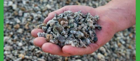
The inherent characteristics of granite mean that ENVIROC® is one of the most versatile and consistent secondary construction aggregates available. We are able to make and supply the vast majority of typical aggregate products including armour stone, type 1 sub-base, 6F5, single sizes, coarse sand, mortar sand, etc.
