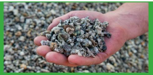
The inherent characteristics of granite mean that ENVIROC<sup>®</sup> is one of the most versatile and consistent secondary construction aggregates available. We are able to make and supply the vast majority of typical aggregate products including armour stone, type 1 sub-base, 6F5, single sizes, coarse sand, mortar sand, etc.
