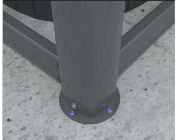
FIGURE 52: ANCHOR THE JACKS TO THE FOUNDATION
