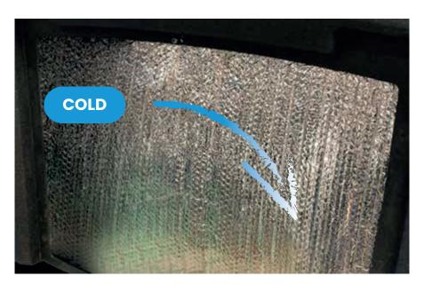
Your *Orion* is extremely well insulated with Thermofoil Blanket. Thermofoil Blanket is reflective and it creates a barrier to contain heat within its walls. The inner walls of the *Orion* are completely covered, floor to top rail, with Thermofoil Blanket insulation.
