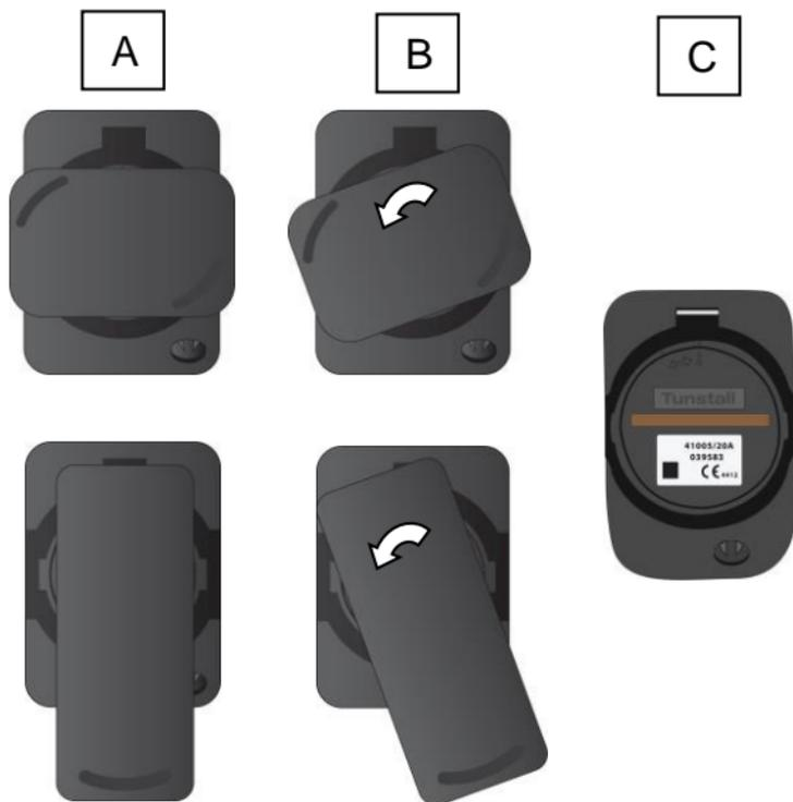
2) Remove the battery cover, insert a well-fitting round coin into the slot and turn it anticlockwise.
