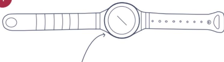
Stretch the wrist strap central circle over the recess in between the front and rear of the button case, it should fit snug without any protrusion
