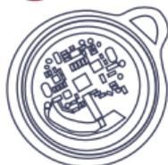
Unscrew & remove the rear of the button case by rotating it anti-clockwise
