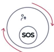
Re-screw the case rear onto the front button case making sure it's tight
