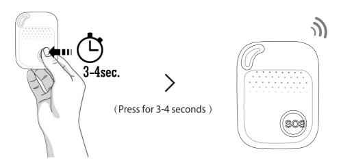
To activate your alarm in an emergency simply hold down the SOS button for 3 seconds until you feel it vibrate. Your alarm will play a pre-alert that allows you to cancel the alarm if it is an accidental activation.
