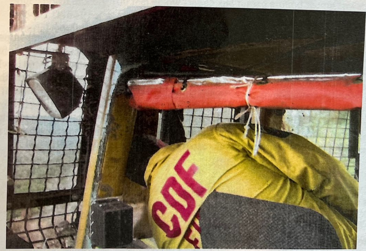
Simulated movement within cab of CAL FIRE D4641 during rollover
