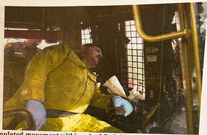
Simulated movement within cab of CAL FIRE D4641 during rollover (Note single lap belt)
