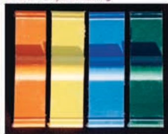
REPNET NET PolyTech Coated™ fiberglass composite posts after the 2,000 hour test.
