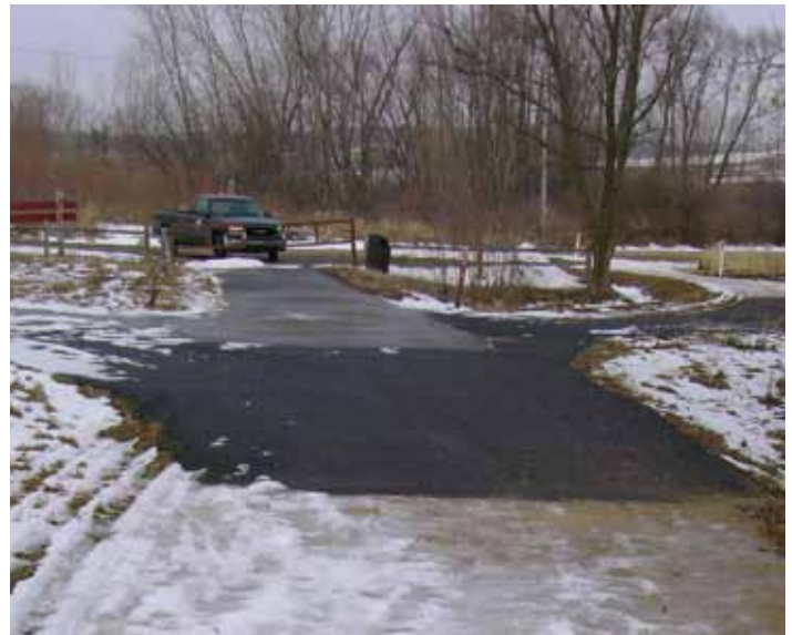
A test section shows how well snow has melted on the porous asphalt section (center) compared to the crushed rock trail (foreground) and regular asphalt (far left and rear)
