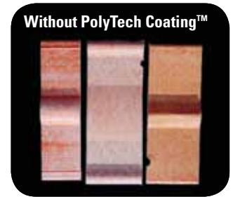
Two competitors' fiberglass posts and our Rhino 3-Rail (left) with clear coat after the 2,000 hour test.
