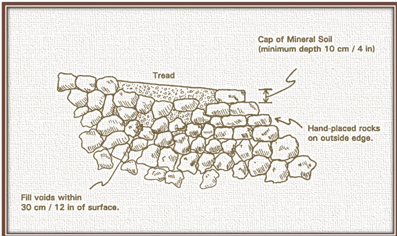
**Illustration 5 - Tread Construction on a Talus Slope**
