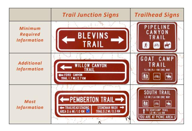
Trailhead signs are metal and rectangular in shape with rounded corners. The sign size should be 45cm x 60cm (18in x 24in). Standard sign colors are reflective-white text, symbols, and border on a brown background. Size of letters and symbols is determined by the best fit to the sign size.
