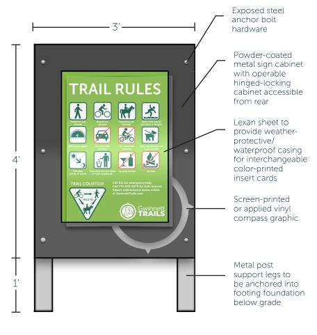
Graphics and text screen printed full color with UV-grade inks on 110 lb. or greater TRAIL RULES paper weight Pictograms and text arranged in grid configuration
