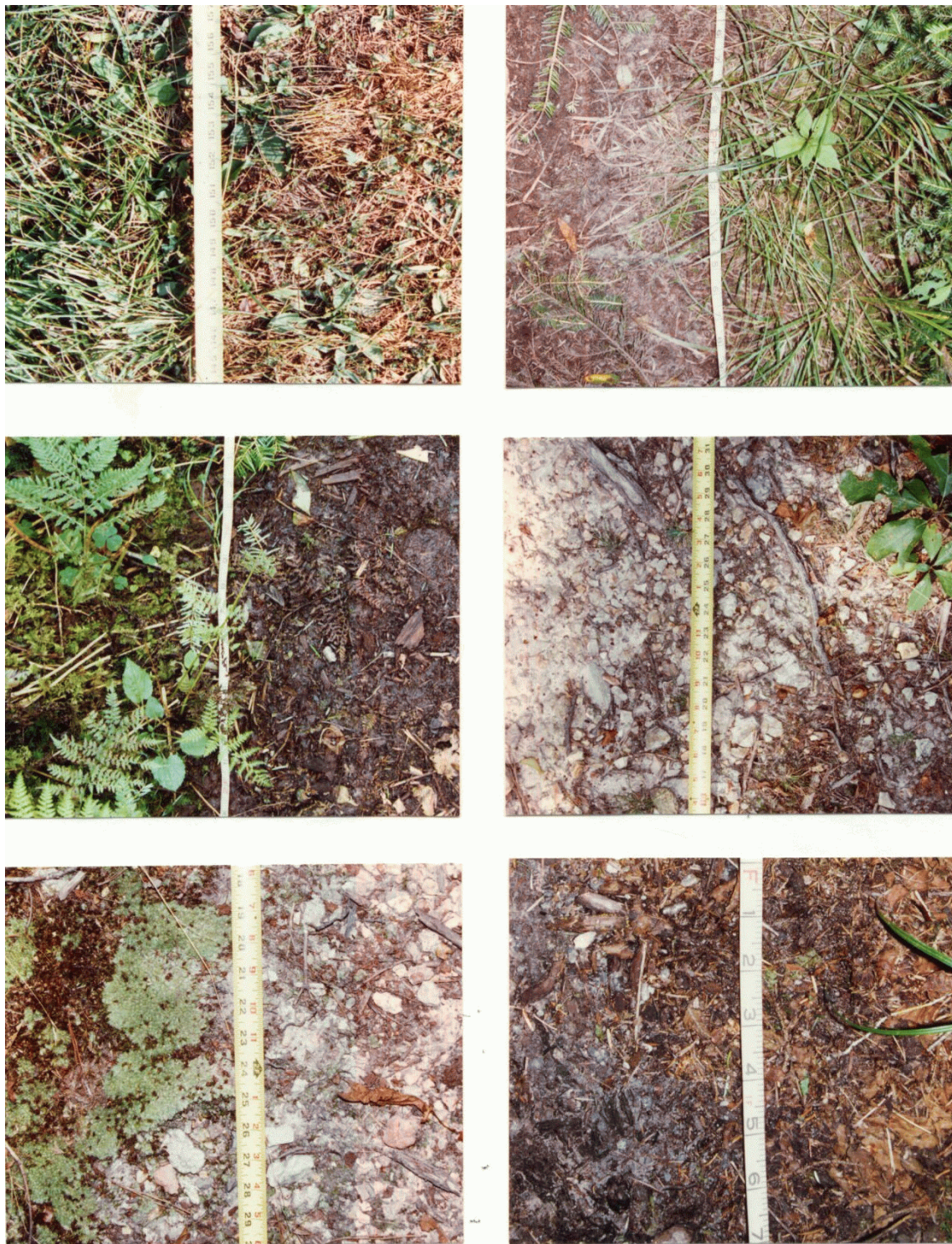
Figure 1. Photographs illustrating different types of boundary determinations. Trail tread boundaries are defined as the most pronounced outer boundary of visually obvious human disturbance created by trail use (not trail maintenance like vegetation clearing). These boundaries are defined as pronounced changes in ground vegetation height (trampled vs. untrampled), cover, composition, or, when vegetation cover is reduced or absent, as pronounced changes in organic litter (intact vs. pulverized). The objective is to define the trail tread that receives the majority (>80%) of traffic, selecting the most visually obvious boundary that can be most consistently identified by you and future trail surveyors.
