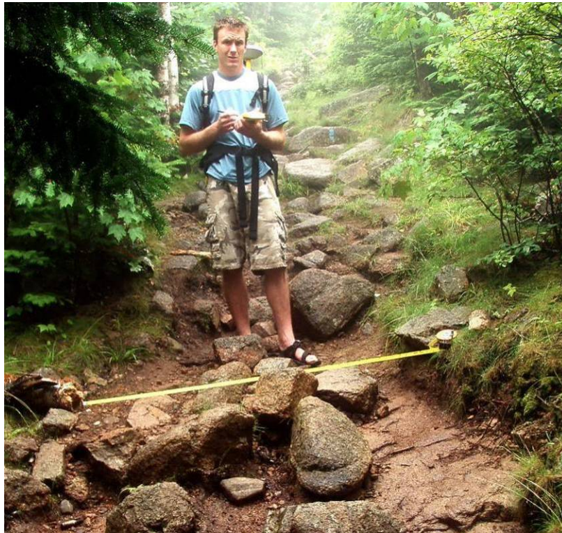
Figure 8. Notice the greater soil loss associated with this fall-line trail alignment compared to the more minimal soil loss for the side-hill aligned trail in Figure 6.
