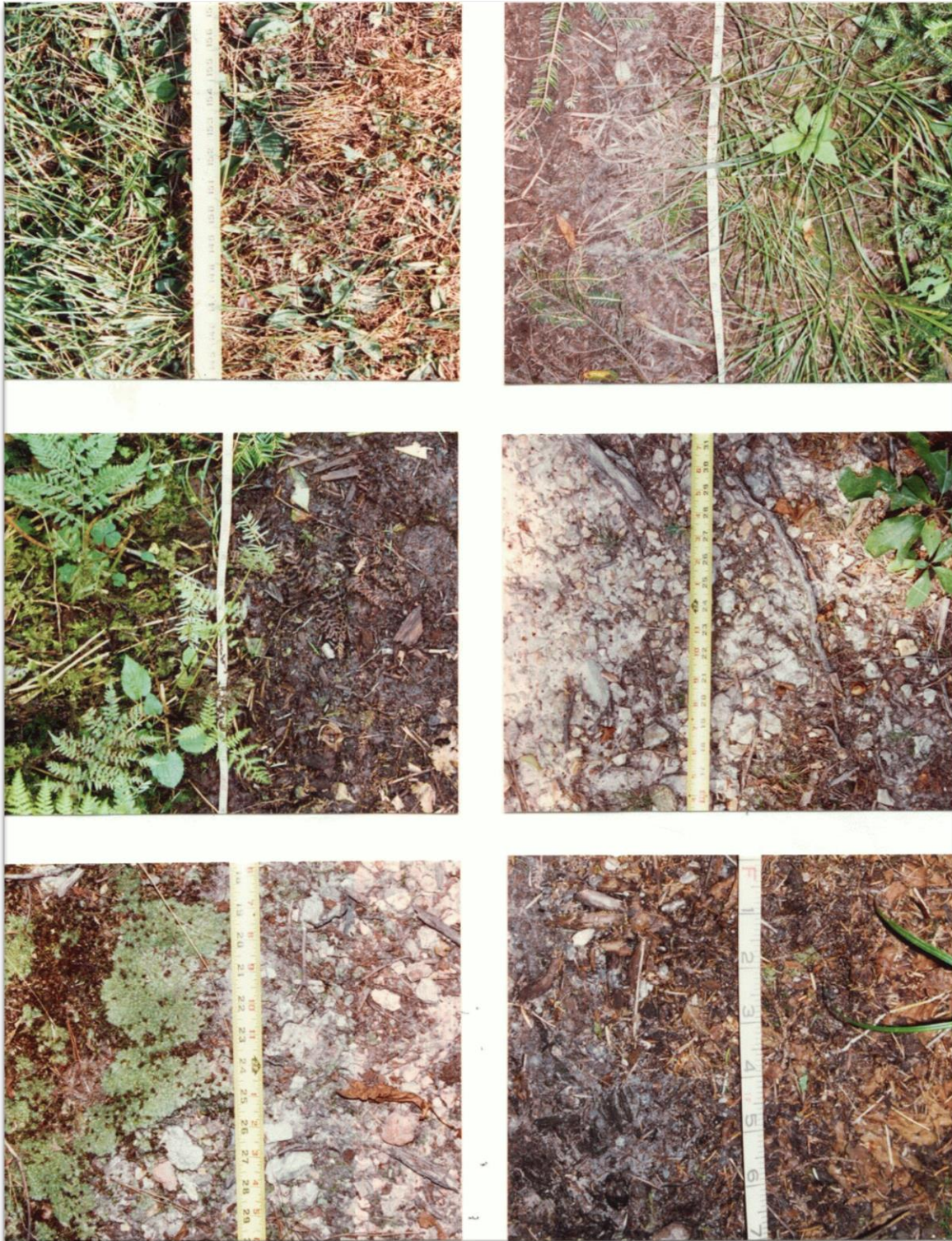
Figure 1. Photographs illustrating different types of boundary determinations. Trail tread boundaries are defined as the most pronounced outer boundary of visually obvious human disturbance created by trail use (not trail maintenance like vegetation clearing). These boundaries are defined as pronounced changes in ground vegetation height (trampled vs. untrampled), cover, composition, or, when vegetation cover is reduced or absent, as pronounced changes in organic litter (intact vs. pulverized).
