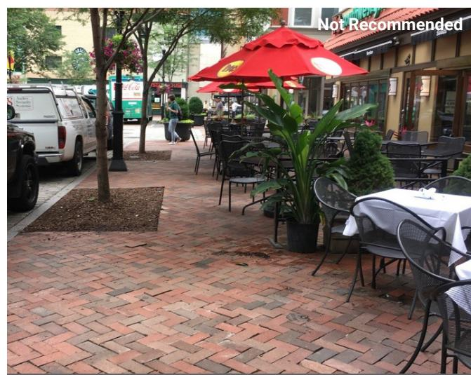
Figure 21: This shared street includes a comfort zone; however, the café seating encroaches on the pedestrian access route and may also encroach on the State Right-of-Way. SOURCE: Accessible Design for the Blind
