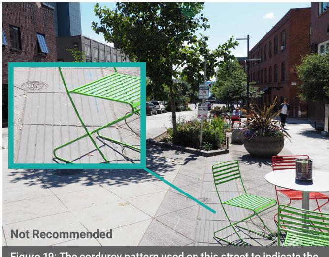
**Figure 19:** The corduroy pattern used on this street to indicate the boundary of the shared zone is not reliably detectable underfoot or by cane and does not provide enough visual contrast with the adjoining surface.
