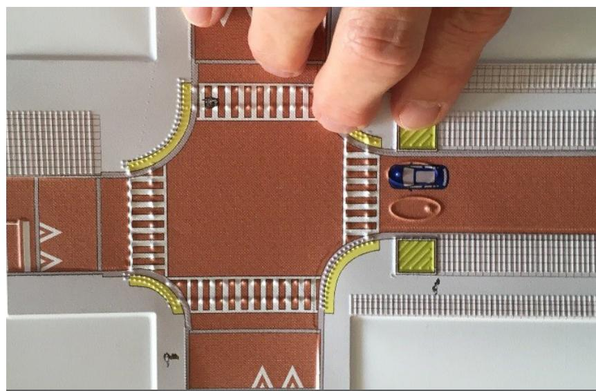
Figure 15: Example of a tactile map showing design of a shared street. SOURCE: Accessible Design for the Blind
