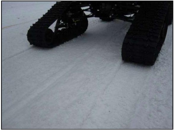
Photo 20: OHV 3 (John Deere Gator 825 UTV) impressions from aggressive stop
