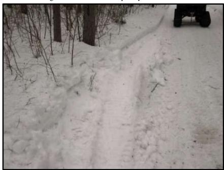
Photo 28: Tracked OHVs were able to operate okay with one track off the compacted trail base
