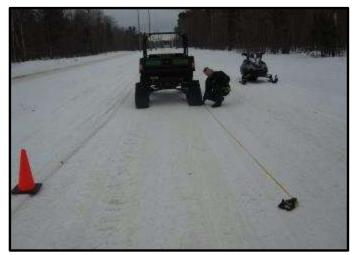
Photo 27: Measuring Vehicle Stopping Distance
