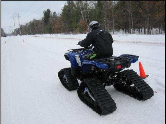
Photo 6: OHV 1 (ATV) Yamaha Grizzly 700 with Camoplast tracks, rear view
