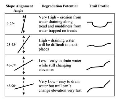
Figure 1. Trail erosion potential and probable profile for trails with different slope alignment angles (landform slope is dotted line/trail is solid line).
