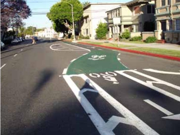
Above and below are two examples of through bike lanes indicating where bicyclists should shift over to allow motor vehicle left turns along the Long Beach cycle track.
