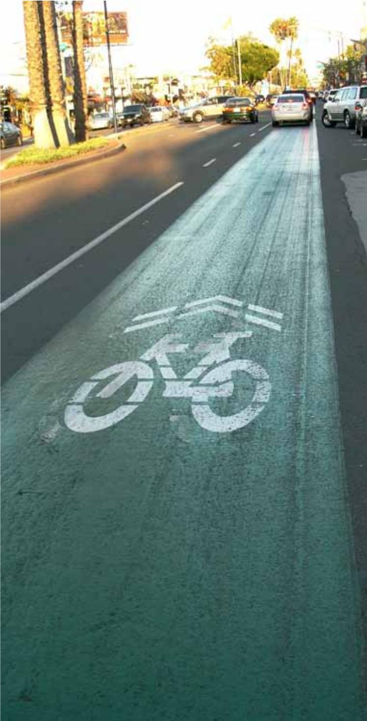
**The green sharrow lane** consists of roadway markings used to indicate a shared lane environment for bicycles and motor vehicles. It is a combination of standard sharrow markings with a continuous green stripe to emphasize the legal right of bicyclists to take the lane. The green sharrow lane is an excellent educational tool that defines the proper location for bicyclists to ride in a shared lane and alerts roadway users to the presence of bicyclists.
