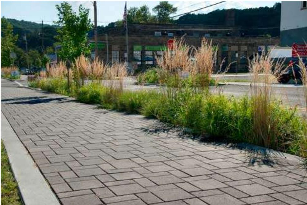
**Permeable pavers and bioswales improve stormwater management.**
