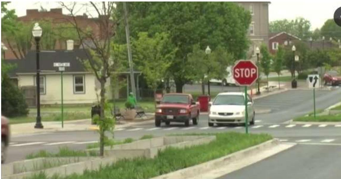
**Median bioswales capture and filter stormwater runoff.**
