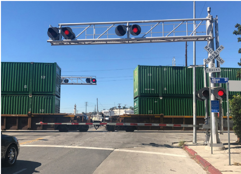
Figure 21. Illustrative Example Showing Cantilever with Flashing-Light Devices
