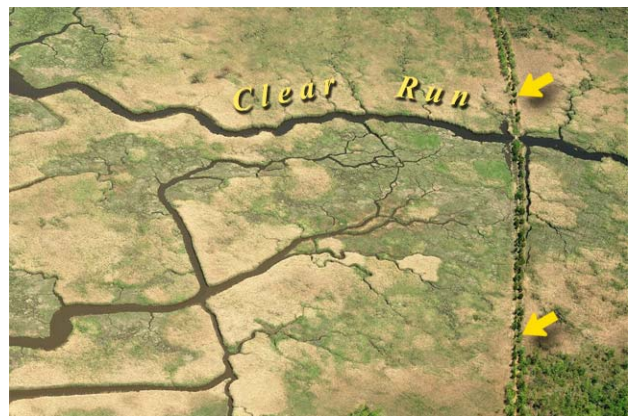
Winchester & Western railroad was built on berm parallel to the east shore of the Maurice River
