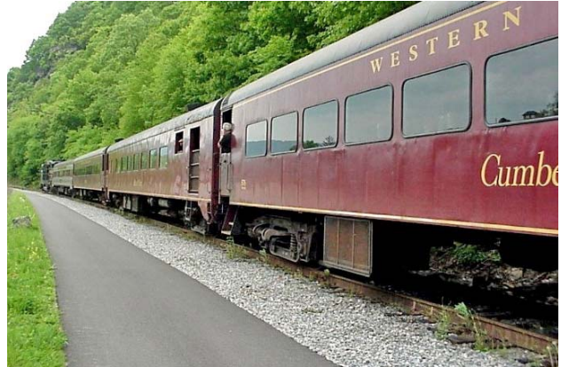
When just one track is abandoned of a double-track railroad, there is room for a multi-use trail
