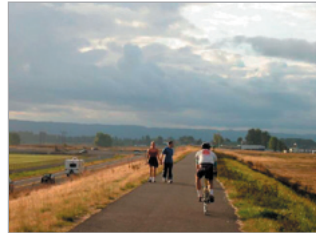
Marine Drive Trail near the airport - stormwater runoff from asphalt infiltrates on grassy side slopes
