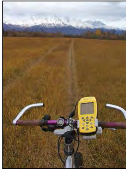
Figure 9–5—This handlebar-mounted Global Positioning System unit was used for centerline data collection on a pioneered off-highway vehicle trail. The use of a mountain bike allowed for quick data collection with little additional environmental impact.
