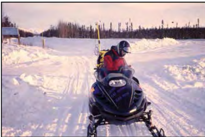
Figure 9–4—Global Positioning System centerline mapping of off-highway vehicle trails may be conducted in the winter by snowmobile. This technique can provide for very rapid data collection in some areas.
