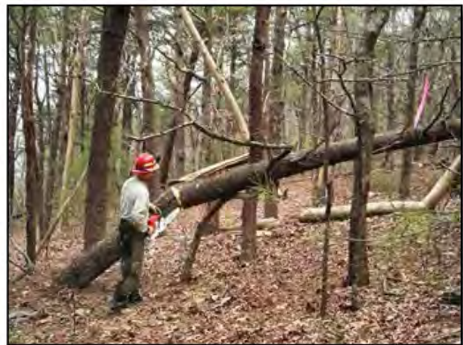
Figure 14–5—Job hazards vary by project task. The hazards associated with chain saw use are different than operating equipment, working on a construction line, or conducting a helicopter sling operation. Note the use of appropriate personal protective equipment for this sawing operation—hardhat, gloves, chaps, and ear and eye protection.
