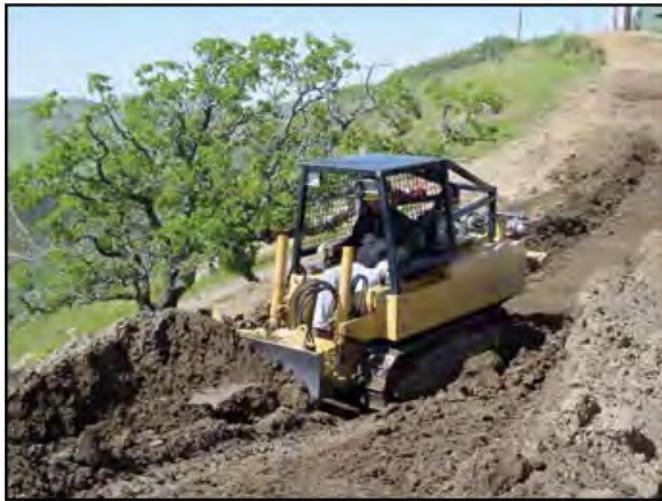
A Sweco 480 trail dozer similar to the one used to construct the Compeau Trail. The Sweco 480 is a 4-foot-wide machine with a 5-foot-wide blade.
