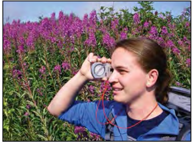
Figure 10–1—A clinometer is used to measure trail grade. This small hand-held instrument allows trail grade or terrain sideslope to be measured quickly and easily.
