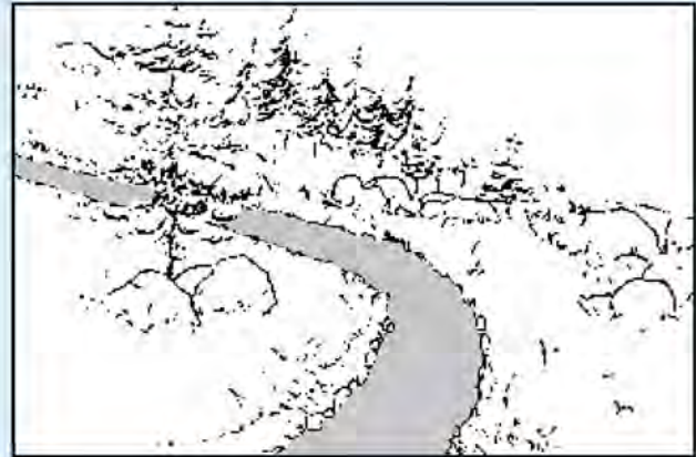
Figure 12–4—Climbing turns continue the climb throughout the turn, and they should be insloped. Add grade reversals at both approaches to keep water off the turn.
