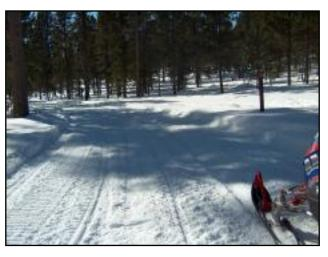
degrees curve were 3 to 4 cm (1.2 to 1.6 in) deep and 41 **Photo 79: Surface chew from snowmobile pass-bys** to 45 cm (16.1 to 17.7 in) wide. There was significant snow spray from the track during uphill acceleration.
