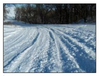
aggressive runs). The snowmobile's track was displacing/ Photo 55: Impressions from a fast pass-by spraying surface snow versus digging snow from the compacted trail base.
