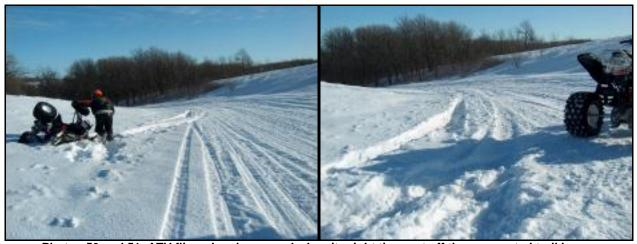
Photos 50 and 51: ATV flipped end-over-end when its right tires got off the compacted trail base
