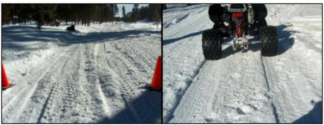
Photo 63: Impressions and piles from a fast start
