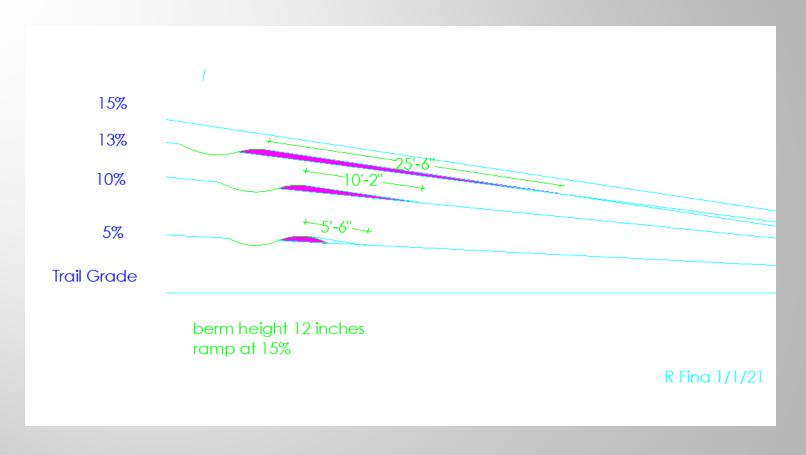
Grade dips work well on trail up to about 15% tread grade, after that the ramp down the back side starts getting too steep.
