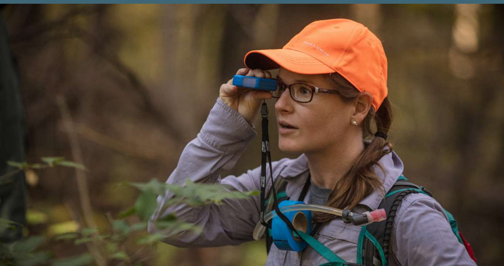
Trail builder using a digital clinometer for measuring slopes and determining trail grades in the field at a project in Chattanooga, Tennessee. Photo by Chrisman/IMBA
