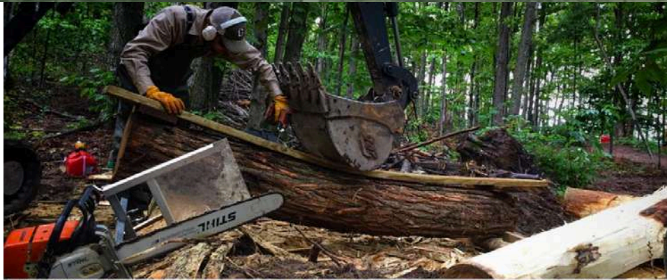
Portable chainsaw mill for planing logs in the field. Photos by Chad Landowski/Traction Trailworx
