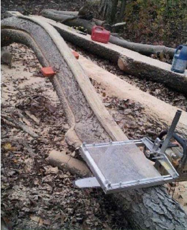
Portable chainsaw mill for planing logs in the field. Photos by Chad Landowski/Traction Trailworx
