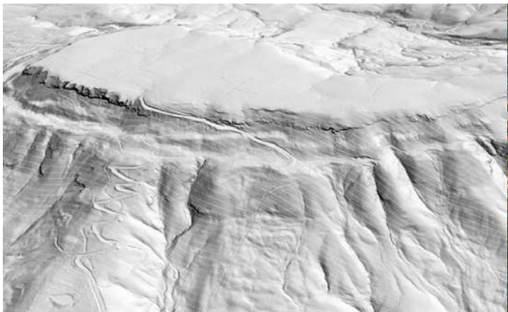
GIS hillshade model used to assess terrain characteristics. Image courtesy of Rock Solid
