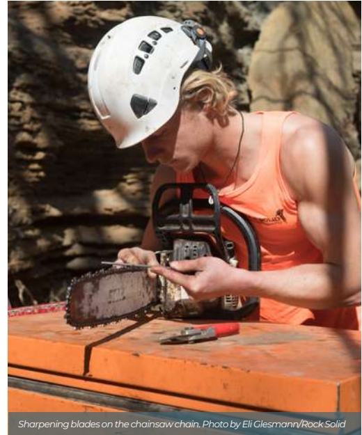
Sharpening blades on the chainsaw chain. Photo by Eli Glesmann/Rock Solid
