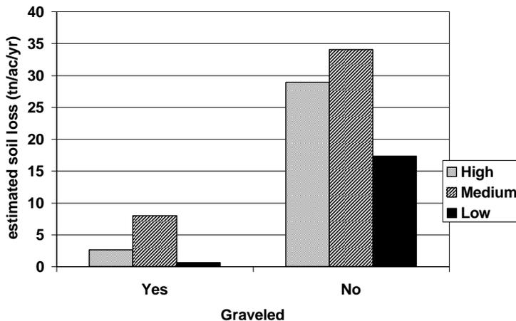
Figures 10 and 11 illustrate the effects of gravel and use level on USLE and CSA levels, respectively. The beneficial effects of gravel are obvious, but interestingly, estimated soil losses are greater from the moderate use trails as opposed to the high use trails. This might indicate that moderate use trails receive less reconstructive or maintenance attention than do the high use trails.
