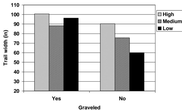
Graveled horse trails are wider than trails with bare soil surfaces (Figure 13). This likely reflects the method of application or that gravelled trails were wider to begin with due to former uses. Note that the surface condition effect varies with level of use. Differences are greater with decreasing level of use.
