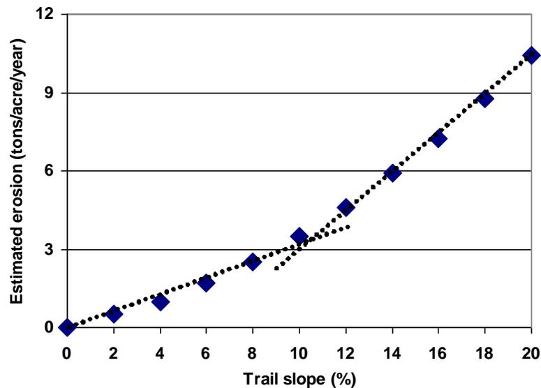
Figure 6. Effect of trail slope percent on estimated erosion if rainfall and runoff factor ( $R = 175$ ), soil erosivity ( $K = 0.3$ ), slope length ( $L=100$ ) and cover and support practices ( $CP = 0.04864$ ) are held constant for the USLE (Dissmeyer & Foster 1984). Note that the effect of slope becomes more pronounced after 10-12 % slope. (Dashed lines are for visual emphasis)
