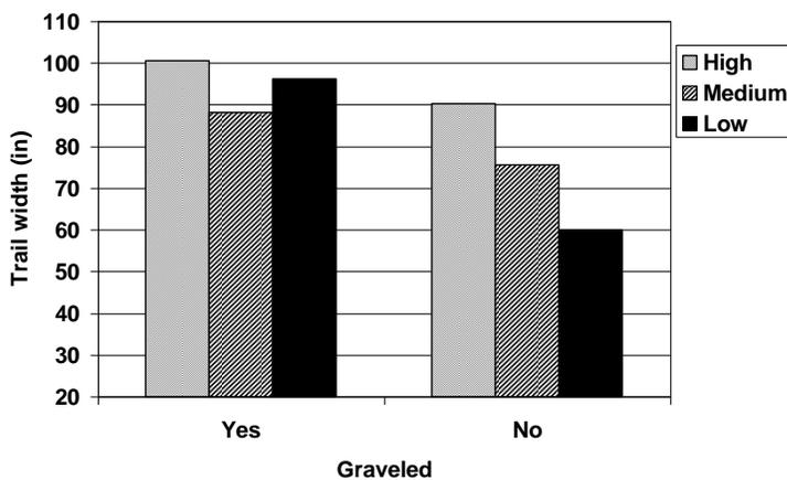
Gravelled horse trails are wider than trails with bare soil surfaces (Figure 13). This likely reflects the method of application or that gravelled trails were wider to begin with due to former uses. Note that the surface condition effect varies with level of use. Differences are greater with decreasing level of use.
