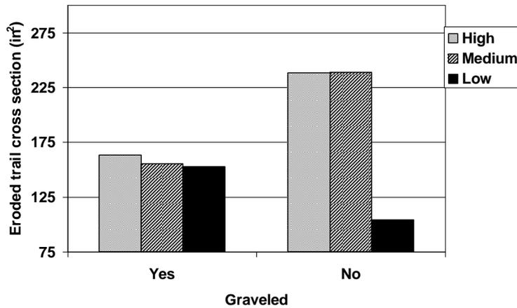
Graveled trails are less eroded than non-graveled trails at the moderate and high use levels (Figure 11). At the low use level gravelled trails had more erosion, hence the significant interaction effect in Table 12. This difference at the low use level cannot be explained and may be attributable in part to the smaller sample size of gravelled low use trails (N=41 points).
