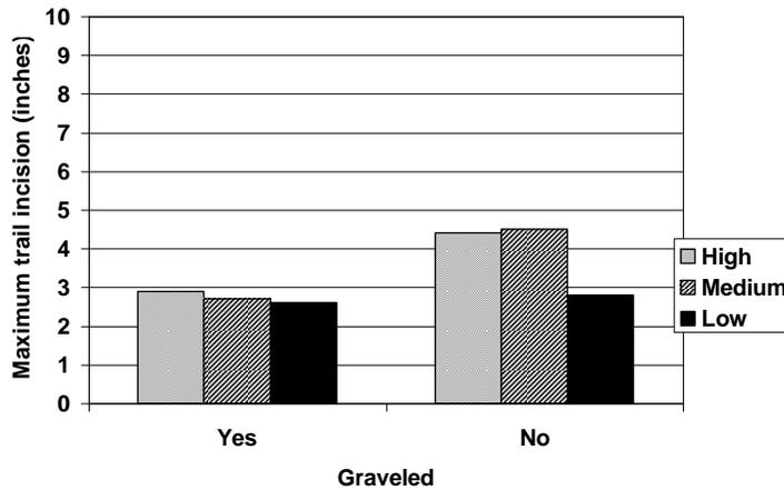
Mean maximum incision values are lower for gravelled horse trails only at the high and medium use levels (Figure 12). At the low use level differences are minor and not statistically significant.
