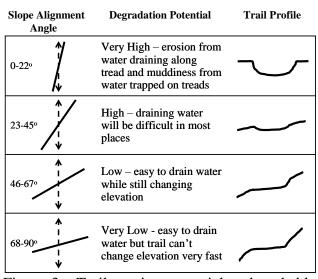
Figure 3. Trail erosion potential and probable profile for trails with different slope alignment angles (landform slope is dotted line, trail is solid line).
