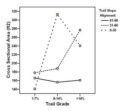
Figure 15. Effect of trail grade and trail alignment angle on CSA.
