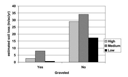
Figures 10 and 11 illustrate the effects of gravel and use level on **USLE** and **CSA** levels, respectively. The beneficial effects of gravel are obvious, but interestingly, estimated soil losses are greater from the moderate use trails as opposed to the high use This might indicate that moderate use trails receive less reconstructive or maintenance attention than do the high use trails.
