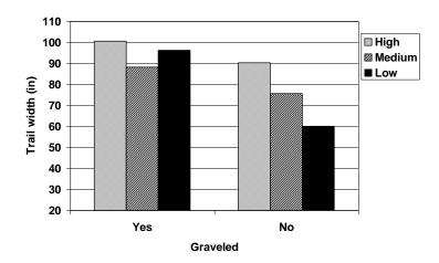
Graveled horse trails are wider than trails with bare soil surfaces (Figure 13). This likely reflects the method of application or that graveled trails were wider to begin with due to former uses. Note that the surface condition effect varies with level of use. Differences are greater with decreasing level of use.
