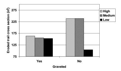
Graveled trails are less eroded than non-graveled trails at the moderate and high use levels (Figure 11). At the low use level graveled trails had more erosion, hence the significant interaction effect in Table 12. This difference at the low use level cannot be explained and may be attributable in part to the smaller sample size of graveled low use trails (N=41 points).
