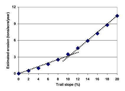
Figure 6. Effect of trail slope percent on estimated erosion if rainfall and runoff factor (R=175), soil erosivity (K=0.3), slope length (L=100) and cover and support practices (CP=0.04864) are held constant for the USLE (Dissmeyer & Foster 1984). Note that the effect of slope becomes more pronounces after 10-12 % slope. (Dashed lines are for visual emphasis)
