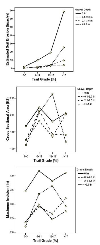
Figure 14. Effect of trail grade and gravel depth on USLE, CSA, and maximum incision.
