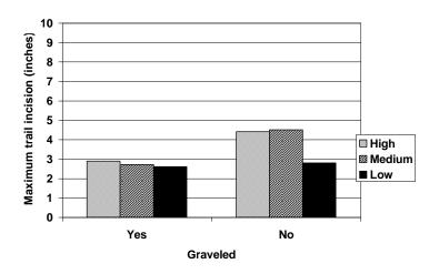
Mean maximum incision values are lower for graveled horse trails only at the high and medium use levels (Figure 12). At the low use level differences are minor and not statistically significant.
