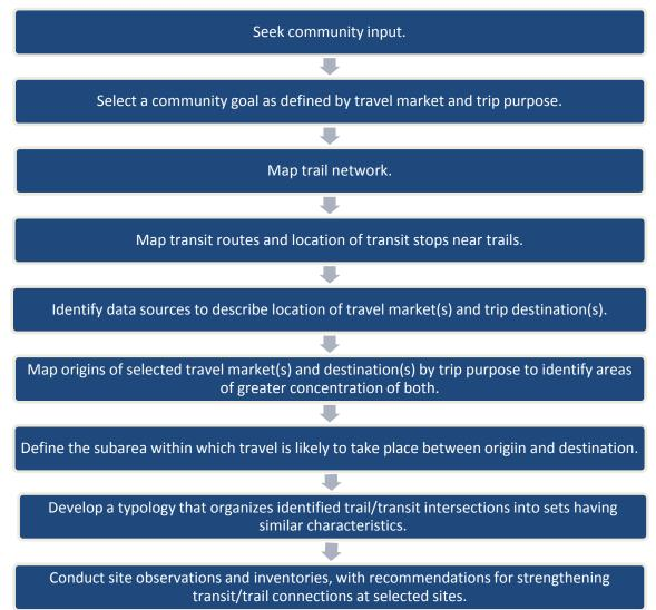
Figure 4: Steps in the method for linking greenways and trails with public transportation
