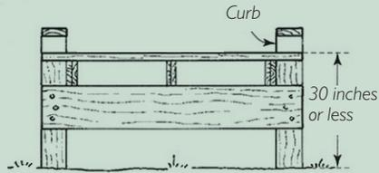
As a general rule, a handrail is required whenever the deck height of a boardwalk or footbridge exceeds 30". A curb can also be added to alert users of the edge of the deck and add character.
