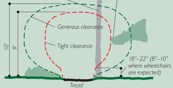
Clearance zones are average distances. Individual tree trunks, branches, etc. can optionally extend to the tread edge. Width varies by use and desired trail experience.
