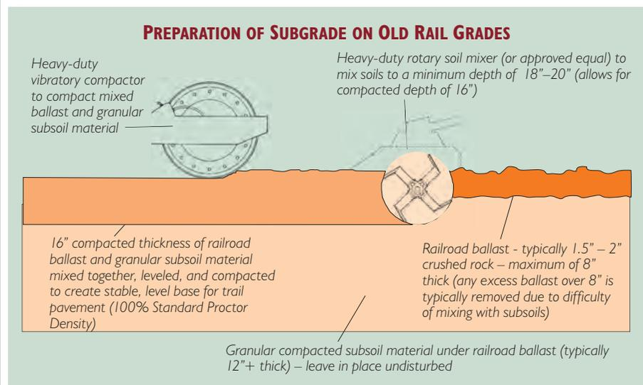
When the rail grade is prepared, the pavement design is consistent with that used for sand and gravel subsoils (above).
