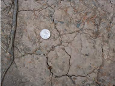
*Silty clay is firm when dry but slippery when wet. The quarter provides a sense of scale.*
