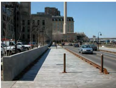
*In an urban setting, hardscape can be used to reinforce where trail users should be. Texture changes, bollards, and retaining walls are some of the features that can be used to control flow while actually enhancing the experience.*
