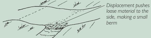
**3. Sediment fills in behind the berm.** In dry conditions, the continued flow of displaced material from above fills in behind the berm. With runoff water, material fills in behind the berm dam, slows there, and settles out. Many small rains can slowly build up layers of sediment that raise and level out the dip bottom inside the tread.
