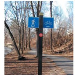
Small, simple signs alerting trail users to which side of the path to use are appropriate at access points or wherever the trail configuration changes. The character of these signs should be consistent throughout the system to make reacting to them second nature to the trail user traveling at different speeds.
