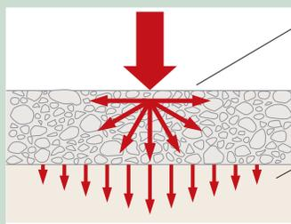
Increasing the aggregate thickness spreads the load over an increasingly wide area.
