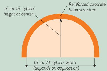
Bebo-type arched structures are used when a larger underpass is needed for trail uses. The height and width of the structure are greater than a traditional box culvert to allow adequate space for maintenance vehicles under the arch.
