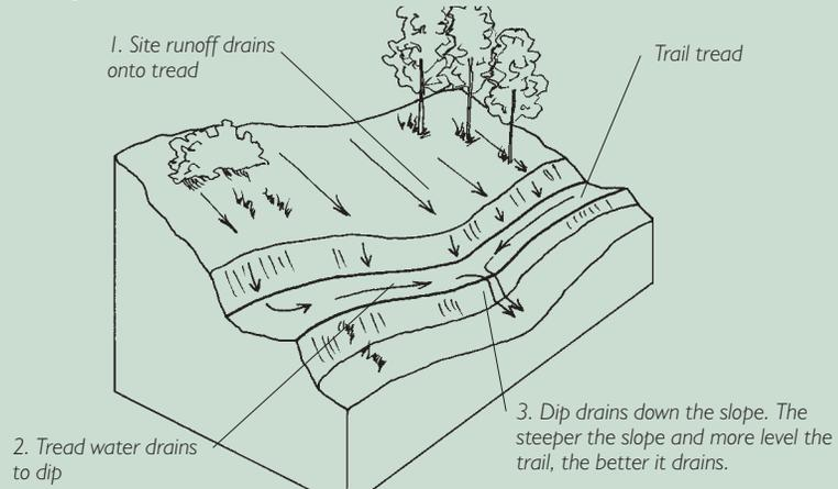
A trail using rolling grade can still climb a hill as long as the climb is not continuous, as illustrated below.
