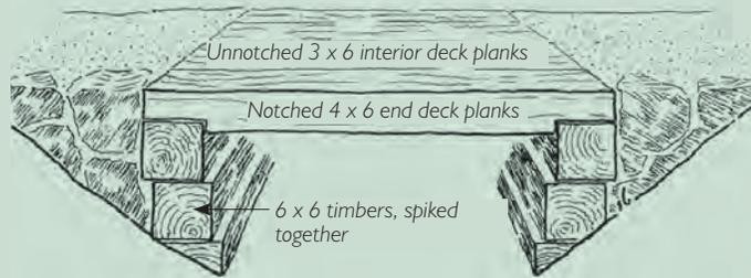
Treated timbers are occasionally used for culverts along natural surfaced trails. Notching the deck planks on both ends helps to brace the walls. Two planks with notches are adequate for a wall up to 24 inches high.
