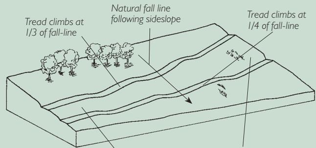
Note that the sideslope is slight on the left but steeper on the right. This enables both trails to climb at a faster rate on increasingly steep slopes to the right.
