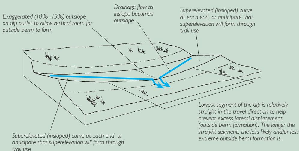
Example of good jogging alignment dip for wheeled uses. The entire dip is long and gentle rather than short and abrupt. The bottom of the dip has an exaggerated outslope and is in a relatively straight segment of the curve. The curve is gentle enough to reduce displacement and user-formed superelevation. The dip has a definite bottom so that if ponding does occur on the tread, it can't spread lengthwise.
