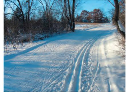
This uphill section does not require much trail widening since it is gentle and short enough for either style of skier to maintain form and make it up with relative ease. This segment retains the recommended 12- to 14-foot width.
