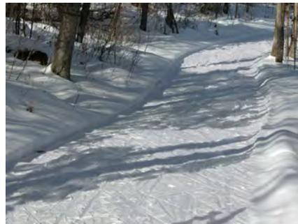
**Skate style - single width/one direction.** These trail are occasionally used in a county, regional, or state park where use pressures are high and/or where separation of skiing styles is preferred. They also occasionally are used as connector trails from one loop to the next. Total width is 8 to 10 feet.
