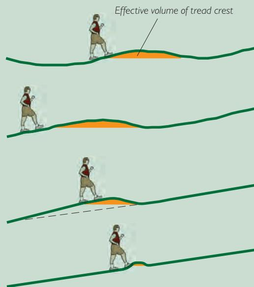
**Crest with near-level trail grade.** The crest is long with a high volume and shallow grades on both ramps up to it. The entire orange area would have to be breached before the crest would fail to separate adjoining tread watersheds. This is very sustainable due to the large size of crest and its intrinsic resistance to displacement.
