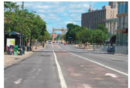
**Center-located bike lane.** On Hennepin Avenue in Minneapolis, the bike lane is located in between traffic lanes going in one direction and bus-only lanes going in the opposite direction.
