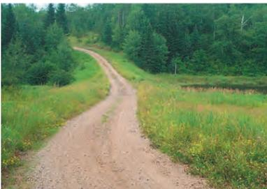
**Wider trail corridor.** On this ATV trail, the corridor includes the buffer area between the trail and ponding area because maintaining healthy natural systems in this area is critical to ensuring the quality of the adjoining wetland and pond system.
