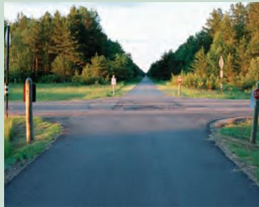
**Standard, easy-to-see at-grade trail crossing in rural area.** This highly visible trail crossing works well in this setting. Although not shown, sightlines from the roadway are open and trail users are easy to see.
