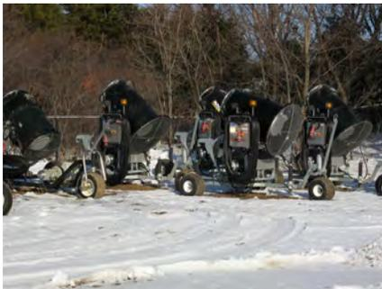
Snow-making equipment is typically portable and is moved along the trail from station to station. Wind and air temperature can greatly affect the quality and placement of the snow as it is created.
