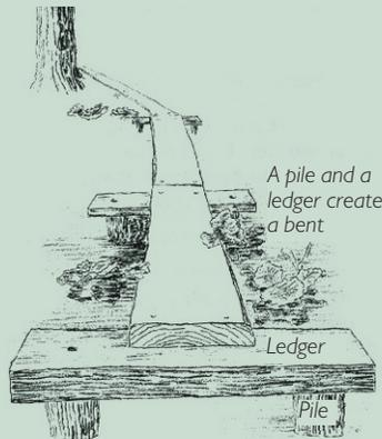
Treated timbers used as piles with either a double ledger (left) or single flat ledger (right) to support a plank tread are commonly used on rustic or remote trails where simplicity is a necessary for ease of construction.
