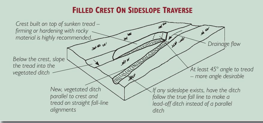
Crest built on top of sunken tread – firming or hardening with rocky material is highly recommended.
