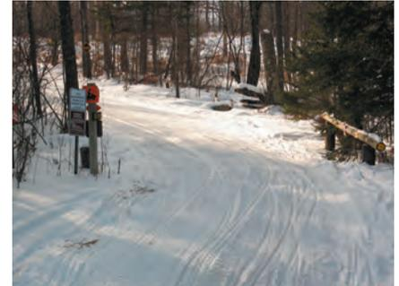
Provide adequate visual cues of an approaching tight curve to enhance trail safety. From this direction, the gate and other signs at the trailhead alert the rider of the approaching curve. From the other direction, a warning sign is provided about 100 feet prior to the curve to alert riders to slow down and approach with caution.
