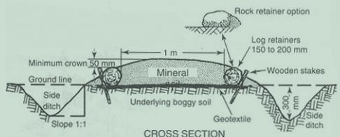
Turnpikes have also been used over the years for crossing wet areas. If this approach is used, caution must be taken to avoid blocking surface water flows or otherwise changing hydrology. If that is likely to occur, a boardwalk is recommended instead.
