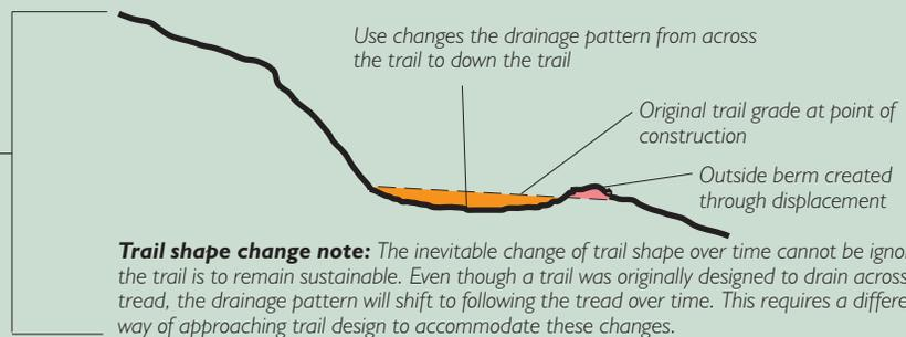
For new or rebuilt native treads, these changes generally occur within a few months to 3–7 years. Timing and the amount of change depend on the tread material, trail use type and levels, and many other factors – but the direction of change is always the same.
