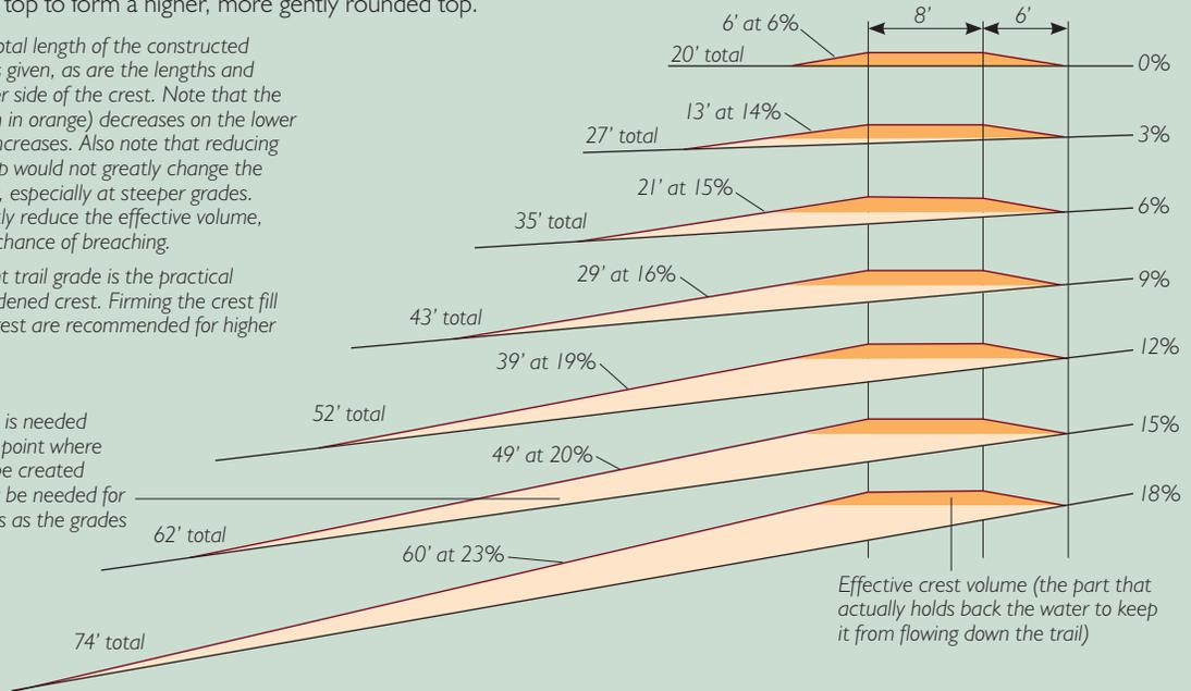
If formed using good techniques, filled crests have more capacity for water handling and often need less maintenance than other forms of constructed crests, such as waterbars. For these reasons, they are generally preferred over other forms of constructed crests. Hardening of the crest can further improve sustainability by reducing the likelihood of displacement.
