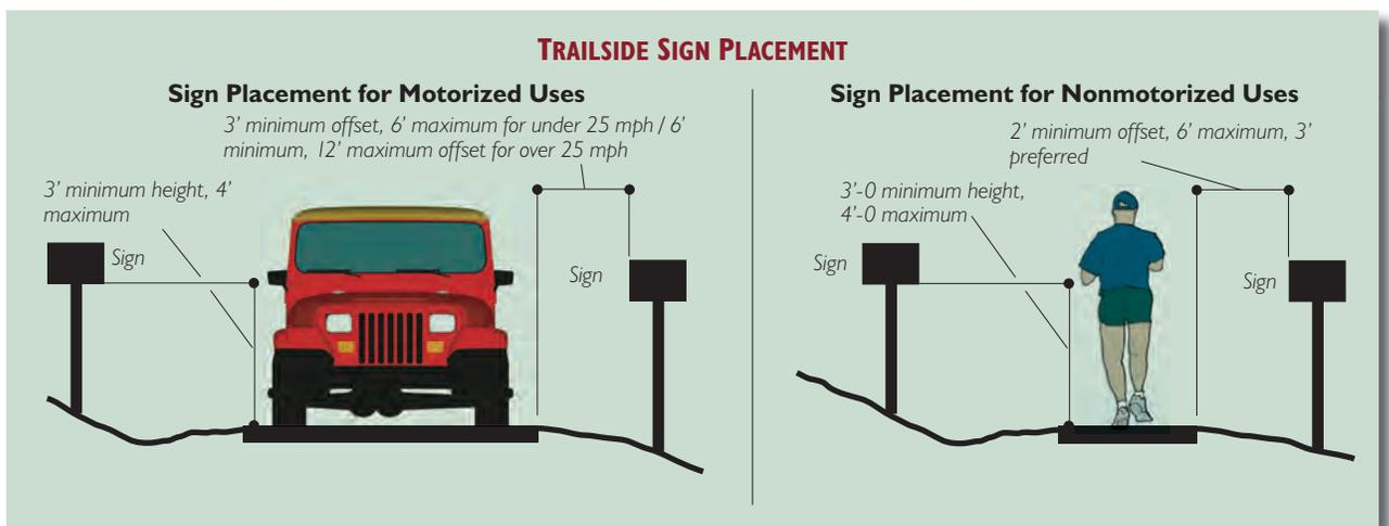
Regulatory traffic signs (e.g., Stop, Yield, Do Not Enter) should be located a minimum of 6 feet back from an intersection. For motorized uses, the recommended distance between a warning sign and an intersection or hazard varies with speed, as the following considers:
