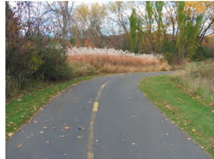
*Paved trails are the least desirable because they do not hold snow nearly as well as grass surfaces. They also are harder on equipment when a bare spot is encountered or the base is too thin.*
