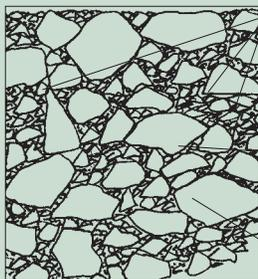
Various sizes of angular particles mechanically interlock into a solid matrix with no voids.
