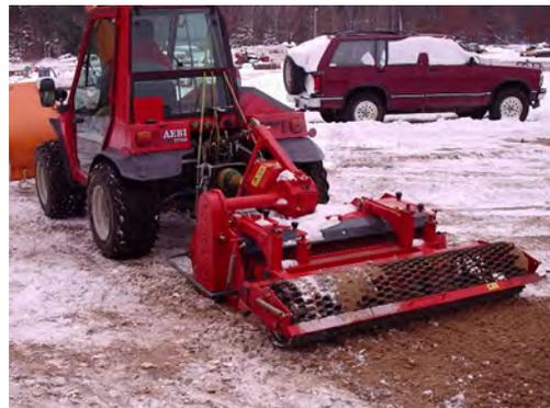
A variety of new implement carriers enter the market each year, each with an extensive array of implement attachments that can till, scarify, blade, level, cultivate, condition, and compact trail surfaces.
