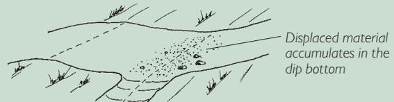
2. **Displacement forms a berm across the dip outlet.** Inside the dip, trail use pushes loose material toward the outside edge. A small berm forms like a dam across the dip outlet.
