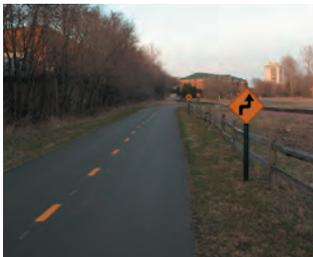
Warning signs alert trail users to a changed condition, such as a curve, narrowing of the trail, or steep grade. Such signs convey an important message and should be consistent with uniform standards. Consistent signing helps trail users' reaction to the signs become second nature and increase their reaction time, resulting in a safer trail experience.
