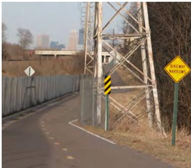
Adequate signage and visual cues alert trail users of the narrowed trail section. Although maintaining a minimum 2-foot shoulder is ideal, that is not always possible in retrofit situations, as is the case with this trail.
