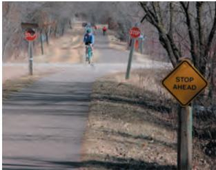
Stop signs are classic warning signs and recommended at all roadway crossings. Note the difference in the size of the sign in these two photos. In general, smaller signs consistent with MN MUTCD standards are recommended for general application and to avoid visual clutter, with larger ones being used to get trail users' attention at more dangerous crossings.
