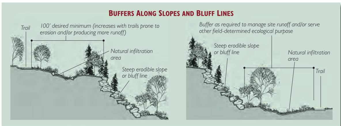
Sometimes a trail must traverse a steep slope. In such cases, it is important to align the trail where site impacts related to stormwater management and erosion can be managed. (Section 6 – Sustainable Natural Trails extensively covers this issue.)
