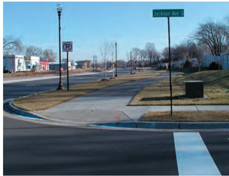
**Landing areas and ramps.** Concrete can be very effectively used to highlight a landing area or accessible ramp where a trail intersects with a street crossing. In these instances, bicyclists and in-line skaters are going slow so the crack control joints in the concrete are not much of a bother. Notably, in the left photo, it is easy to understand how the joints in the concrete would become annoying to trail users over an extended distance.
