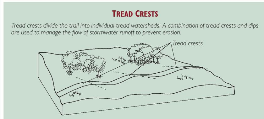
Tread crests are vulnerable to breaching when runoff from one watershed flows through an adjoining crest into the next. The three main causes of crest breach are:
