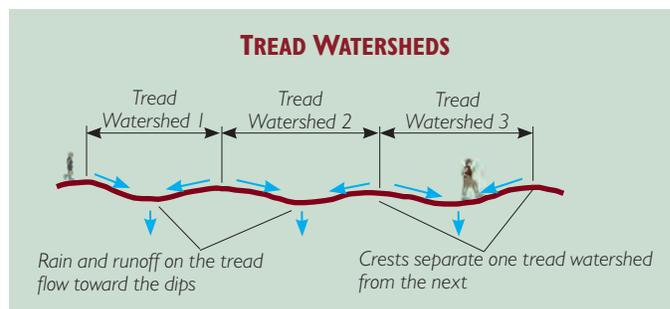
A tread watershed consists of the tread surface plus any uphill area where runoff flows onto the trail and down to a dip between two crests. The only way to prevent erosion is to form tread watersheds so they will not produce enough water to seriously erode the trail. Every dip must also drain to somewhere lower than itself. The most sustainable way to arrange this is by traversing a slope, as the following graphics and accompanying photos illustrate.
