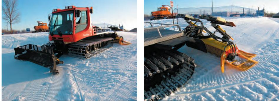
*The Piston Bully is an impressive piece of equipment that can be effective for certain types of conditions, especially moving around artificial snow, which is often heavier and deeper than natural snow. But for most applications, the more economical snowmobile and tow-behind packer and track setter produces excellent results under an experienced operator, especially when snow depths are limited and a larger piece of equipment is excessive.*
