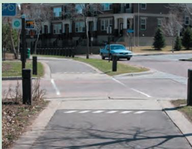
This ramp is as wide as the trail, relatively flat with no significant gutter lip, and protected on each side with bollards. Sightlines are also clean to reduce conflicts with motorists.
