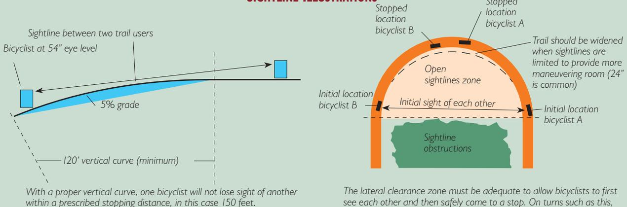
The lateral clearance zone must be adequate to allow bicyclists to first see each other and then safely come to a stop. On turns such as this, the stopping distance for both riders needs to be factored in. Lacking adequate sightlines, trailside warning signs, pavement markings, and pavement widening through the turn are recommended.
