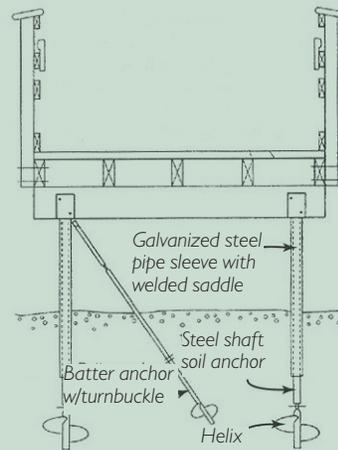
Helical piles (screw piles) are most commonly used where soil conditions make post-hole digging difficult or where minimal grade disruption is desired. Mechanized hand tools can often be used in these instances.
