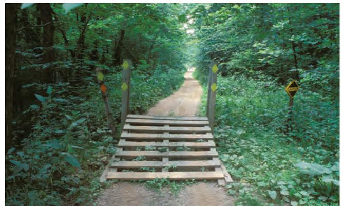
Simple trail structures confining horizontal clearance can create a gateway.
