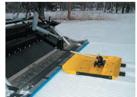
The Ginzu groomer has much in common with the Tidd Tech, with personal preference being the discerning factor on which groomer to use. A combination of weights, springs, and hydraulics are used to increase the level of compaction on the snow surface. One of the Ginzu's strengths is its ability to level out humps and cut hard pack snow.
