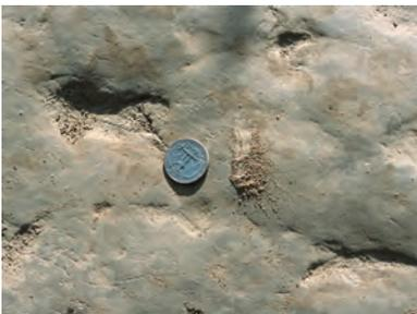
*Loess (windblown mineral silt from glacial grinding) on the Southeast Minnesota ATV Trail becomes so hard in places that the surface is polished with tire marks and is difficult to scratch with a coin. Soil this strong is found only in a few Minnesota locations.*
