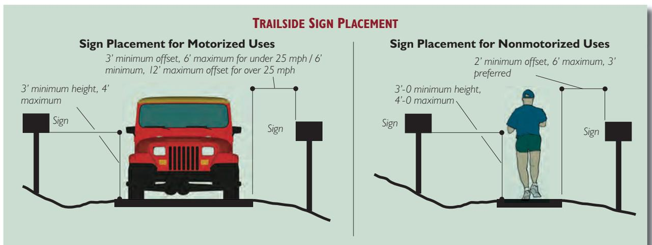
Regulatory traffic signs (e.g., Stop, Yield, Do Not Enter) should be located a minimum of 6 feet back from an intersection. For motorized uses, the recommended distance between a warning sign and an intersection or hazard varies with speed, as the following considers:
