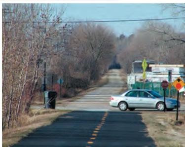
The transition from one surface to another can dramatically change trail speeds. On this trail, travel speeds on the asphalt surface could reach 20 mph. On aggregate, a 12- to 15-mph travel speed is more common.
