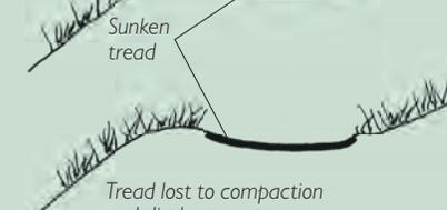
**Inslope partly works.** Tread tends to level into a pan shape which channels water toward its center
