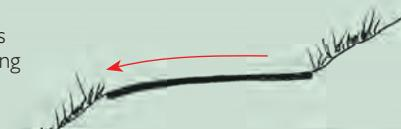
**Inslope.** Tread continually sheet drains to inside while traversing sideslope
