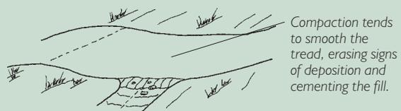
When major storms do occur, flow can be sufficient to fill the outside of the tread. This is more likely where the dip outlet has a shallow grade that causes the dip to fail unless the outlet is cleaned out before the next major rain. It can also happen during a short, heavy rain in which there is enough water to carry sediment into the dip but not enough to flush it through.
