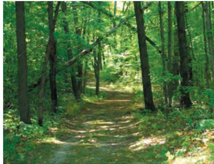
*Although ground cover is sparser along this trail, summer use levels are light enough and the ground hard enough to limit depressions and erosion, making for a very suitable trail surface.*
