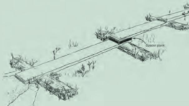
A simple bog bridge with sleepers is a historically common approach to crossing bogs in remote areas with readily available materials. The limitations of this approach is the sleepers will rot out over a period of years and have to be replaced, requiring more maintenance than other techniques.
