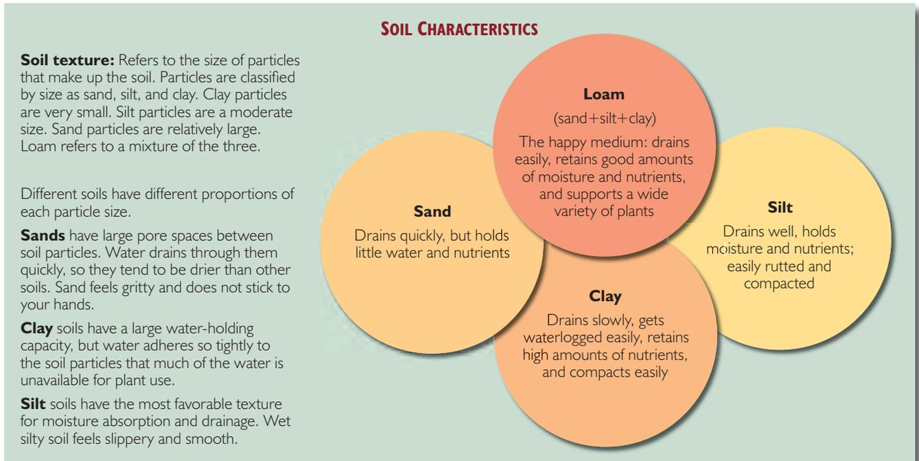
The character of the soil affects the size of the buffer zone needed adjacent to a sensitive ecological system to accommodate natural infiltration. The size and scale of the first two components of the natural infiltration system described on the previous page are most affected by soil types because that is where much of the infiltration is to occur.
