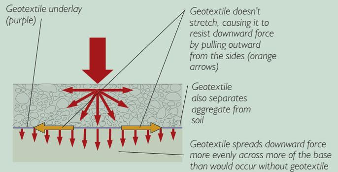
Geotextiles are available in woven and nonwoven forms. Nonwoven forms are preferred because they are easier to handle and spread forces in more directions. Geotextiles will last indefinitely when buried, but are photodegradable and should not be used where they would be exposed to light—including in situations where tread displacement would expose them.
