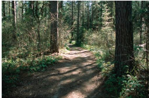
**Compacted tread with gentle grades.** Well anchored by larger trees, this on-road trail has gentle grades in well-drained, sandy-stony soil. The tree canopy and low site runoff help protect the tread.
