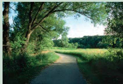
**Adequate shoulders.** Both of these trails exhibit shoulders that provide a margin of safety for trail users. In the left photo, the trail sign is about 2 feet from the edge of the trail, with heavy brush cut back from the trail edge 4 feet or more. In the right photo, the heavy grass edge is cut back about 18 inches to prevent taller weeds from encroaching onto the trail and narrowing it, which is annoying to most trail users.
