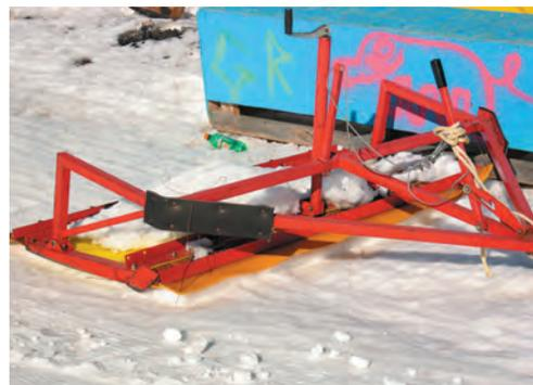
A pan is used to compact and smooth a trail under various conditions. Weights can be added as needed to achieve the desired level of compactness.
