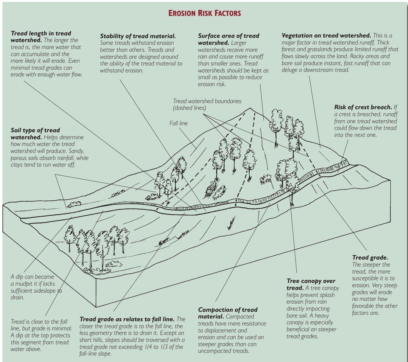
There are two primary ways to minimize the risk of tread erosion: limiting tread grade and limiting the size of the tread watershed.
