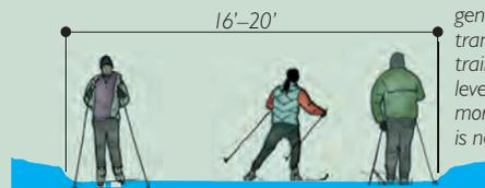
Also used as a linear connector between loops where two-direction use must be accommodated.
