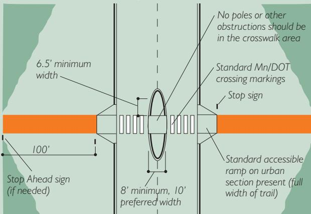
The width of the crosswalk and curb cuts should be 10' minimum. Raised islands should be cut through or have ADA accessible curb ramps with a minimum landing area of 4 feet between ramps.
