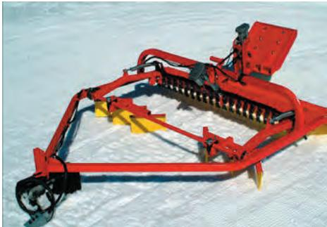
The Tidd Tech groomer (bottom photo) includes a flat pan with a grooved edge to create the desired trail texture for skate-style skiing. The pan can be tilted forward to till or peel up a layer of snow and grind it for repacking. The track setter (top photo) is the last grooming step and sets the track for traditional skiing. It is simply an attachment to the groomer that is lowered to set the track.
