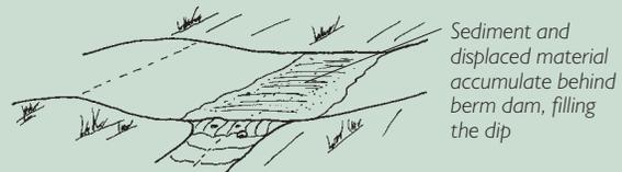
**4. Compaction and water cement the clog.** Since the sediment behind the outside edge berm is in the tread, trail use compacts it. If the material is repeatedly wetted and dried with compaction, it becomes hard and resists erosion. Subsequent runoff through the dip then flows over the compacted, raised tread.
