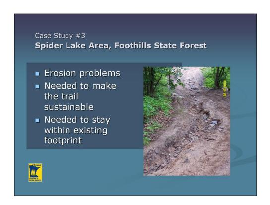
This trail system contains areas with highly erodible soils. Many trail alignments travel the fall line up steep hills which presents a continuing challenge for site manages. Soil stabilization, erosion controls, and stormwater management are very important here. In this case, we needed to harden a climbing turn.
