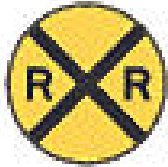
TRAIL-RAILROAD GRADE CROSSING ADVANCE WARNING SIGN
