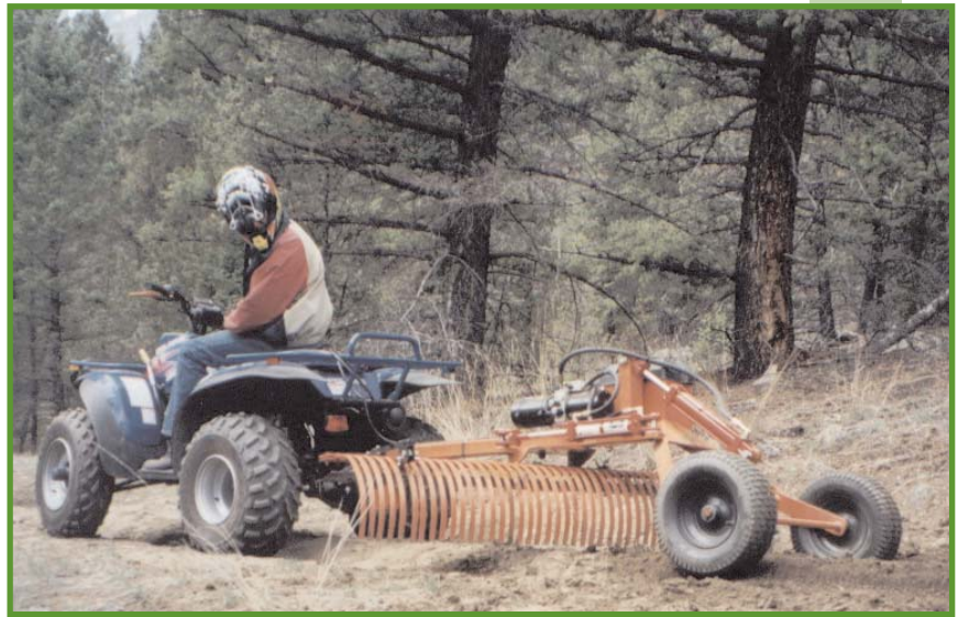
Trail rakes can pull soil from berms without requiring the operator to drive off the trail.
