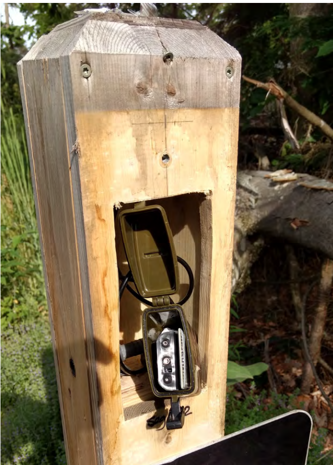
Figure 10-1: An example of a trail counter hidden within a sign post at Sleeping Bear Dunes National Lakeshore in Michigan; sign was turned upside down to expose the counter for the photograph. (Source: NPS)
