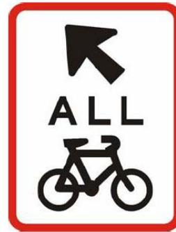
Figure 74: All cyclists must exit regulatory sign (RG-26b) (Transit NZ, 2008b)
