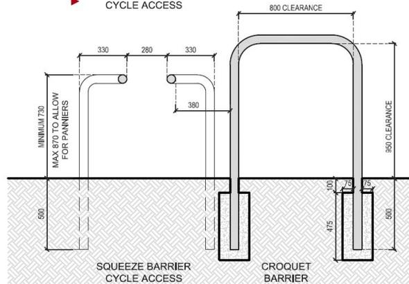
**E** SECTION THROUGH CENTRE-LINE OF SQUEEZE BARRIER.
