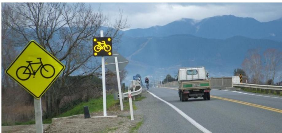
**Figure 39: Inductive loop activated warning sign on narrow Appleby bridge, SH 60, near Nelson (photo: NZTA)**
