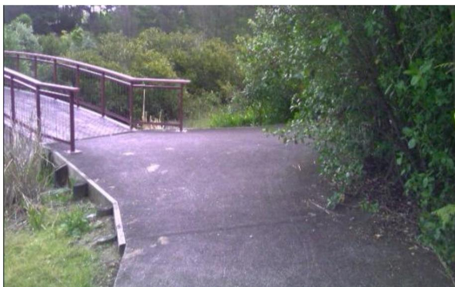
Figure 44: Poor intervisibility at path intersection – Auckland
