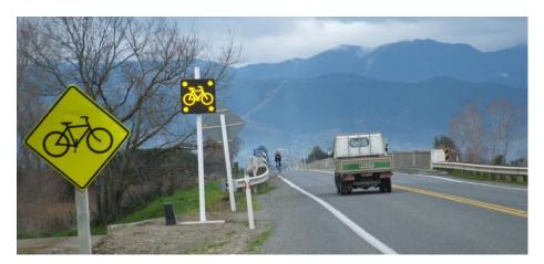
Figure 39: Inductive loop activated warning sign on narrow Appleby bridge, SH 60, near Nelson (photo: NZTA)
