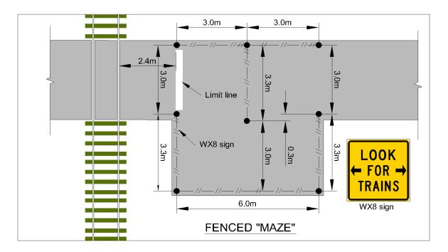
Figure 47: Fenced maze design; slows cyclists before crossing railway line
