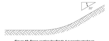
Figure 19: Cross section for Grade 4 superelevated turn
