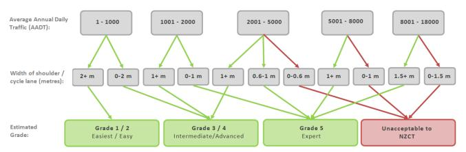
Figure 37: determination of viability of cycle routes on open roads
