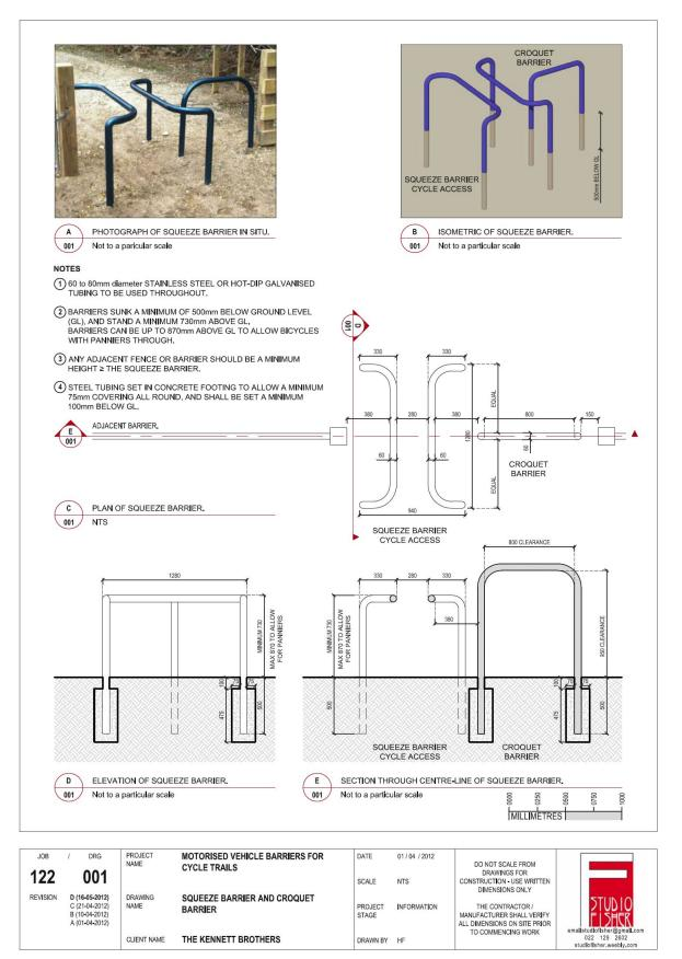
Figure 64: Squeeze barrier and croquet barrier design
