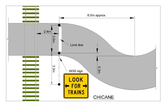
Figure 46: Chicane design; slows cyclists before crossing railway line
