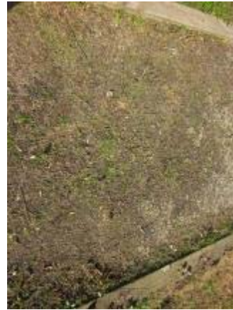
Photo 41 Soiltac Powder Mix-In trail segment with water crossing would soften and then return to natural surface state. November 2, 2011.
