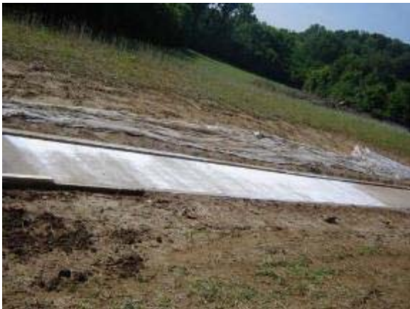
Photo 20 Soiltac Powder Topical has a penetration of \frac{1}{8} inch. June 27, 2007.
