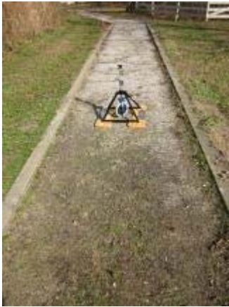
Photo 40 Soiltac Powder Mix-In showed only minor evidence of softening at the end of the study. November 2, 2011.
