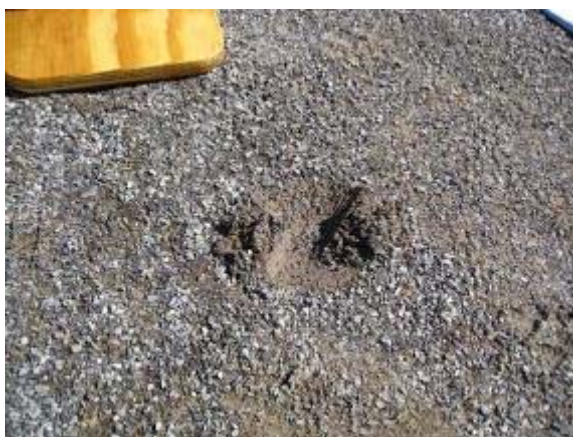
Photo 82 Stabilizer trail segment shows indentation from surface testing. March 13, 2008.
