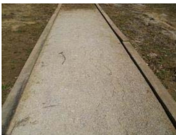
Photo 64 Soiltac Liquid Mix-In trail segment was only slightly soft under foot, showing footprint indentations. March 13, 2008.
