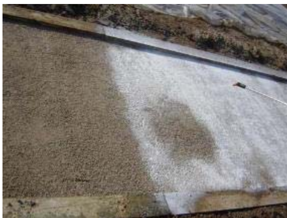
Photo 44 Soiltac Liquid Topical has a penetration depth of \frac{1}{8} inch. June 27, 2007.
