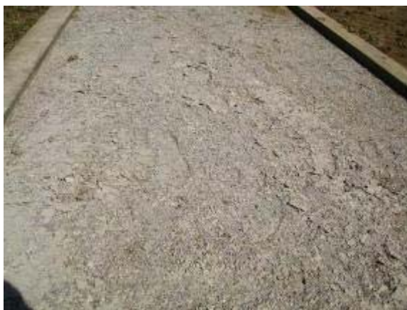
Photo 46 Soiltac Liquid Topical trail segment became soft under foot. March 13, 2008.
