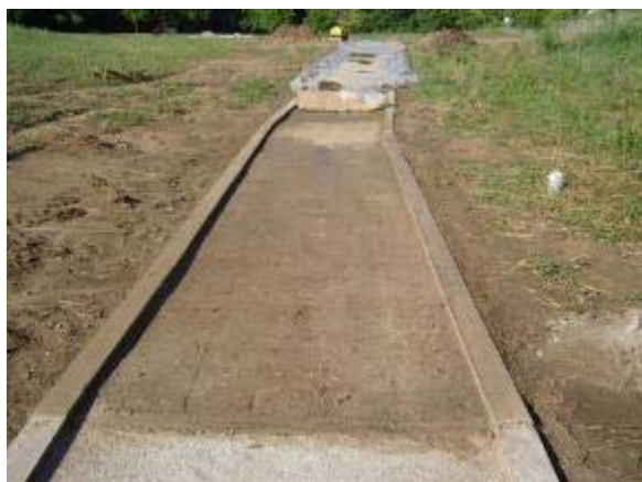
Photo 110 Polypavement trail segment started to show signs of cracking and softening after the first round of tests. July 6, 2007.
