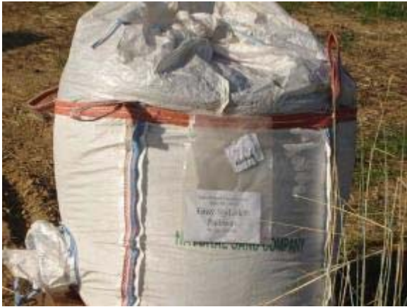
Photo 90 StaLok arrives pre-mixed with 1/4 inch minus aggregate. June 21, 2007.
