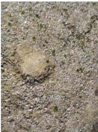
Photo 51 Soiltac Liquid Topical trail segment showed footprints. March 17, 2009.
