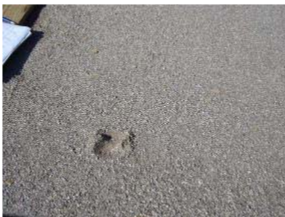
Photo 76 Stabilizer surface shows an indentation from the surface testing. July 6, 2007.
