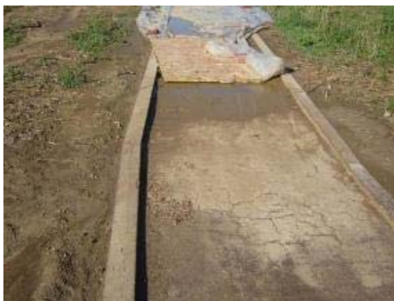
Photo 111 Polypavement trail segment started to show signs of cracking and softening after the first round of tests. July 6, 2007.
