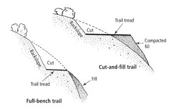
FIGURE 14. Full-bench and cut-and-fill trails provide safe travel across steep slopes. *Drawing courtesy of Baughman and Serres (2006).*
