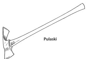
• **Ax.** Look for a long-handled ax to cut tree roots, split wood or cut a felling notch into a large tree. When felling trees or cutting logs, use a saw for greater safety and efficiency. A single-bladed ax with a hammer head on one side can be used to pound stakes and wedges, but a sledge hammer is safer.
