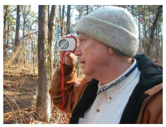
FIGURE 10. A clinometer is a useful tool for evaluating trail grade. *Photo by Becky McPeake, UA Division of Agriculture, Cooperative Extension Service.*
