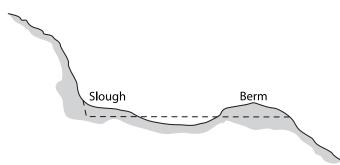
FIGURE 25. Remove the slough and berm, leaving the trail outsloped so water will run off. One fist's worth of drop for the length of a Pulaski is a good rule of thumb.
